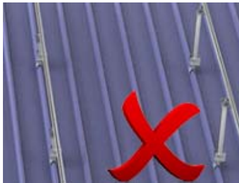
FIGURE 5.2.4.1 EzQuik KLIP-LOK Clamps should never installed parallel to roof ribs
